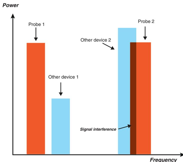
1. Other device 2, with greater transmission power is blocking part of the probe 2 transmission channel.
