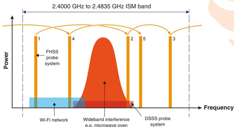
**FHSS probe transmissions co-exist with other radio traffic, while DSSS probe transmissions are compromised**
