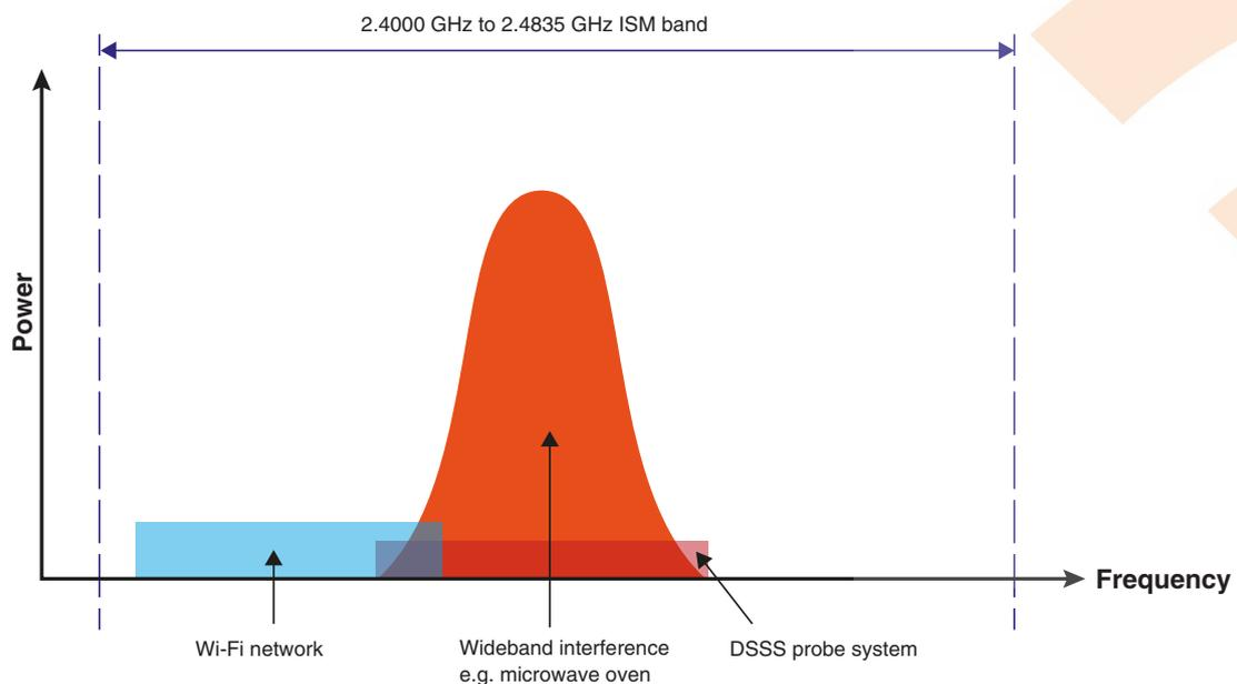
*DSSS probe transmissions compromised by a Wi-Fi network and a wideband interference source*
