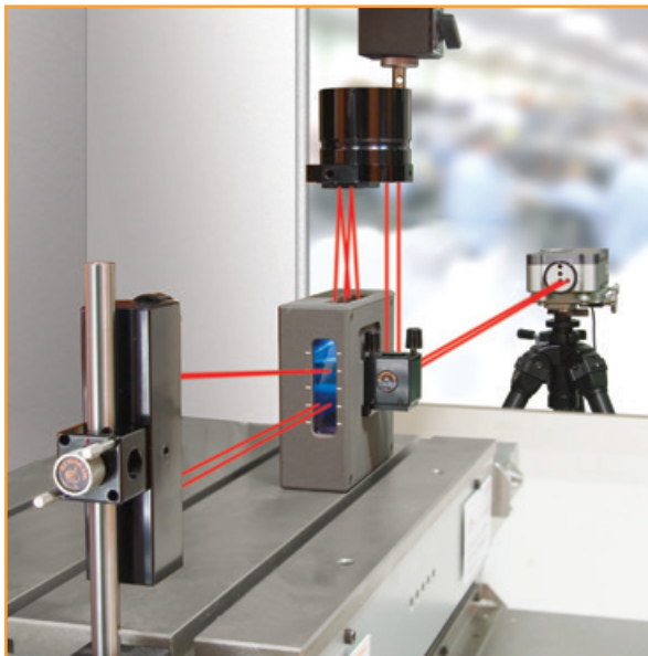
X-Z axis squareness measurement on a VMC
