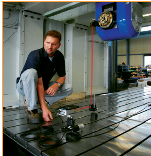
A maintenance and calibration contractor uses XL-80 to verify 5-axis machining centre performance.
